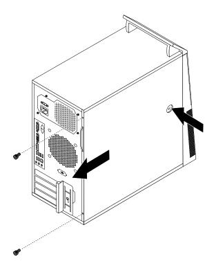
Figure 9. Removing the computer cover
